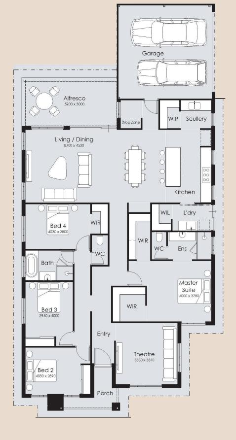
Overall Width – 11.99m Overall Length – 25.29m Min Block Width – 15m Min Block Length – 30m Total Area – 257.97m<sup>2</sup>
